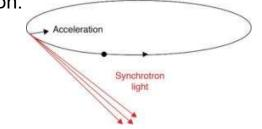
The electromagnetic field surrounding the electrons is unable to respond instantaneously when the electrons are deflected; some of the energy in the field keeps going, producing a tangential cone of synchrotron radiation. As the electrons' energy increases, the cone of radiation narrows, and the radiated power goes up dramatically.
